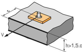
$$\Psi_{s-c,V} = \frac{c}{c_{min}} \cdot \sqrt{\frac{c}{c_{min}}}$$
