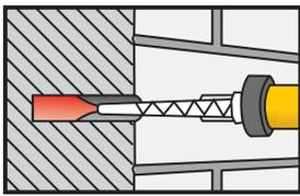
8. Inject the adhesive into the drill hole, starting from the bottom and slowly pull out the static mixer while extruding the resin into the hole. Avoid entrapping air. For deep holes use extension tubing
