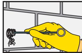
5. The drill hole must be thoroughly cleaned again as stage 3
