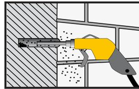
6. The drill hole must be cleaned again as stage 2 & 4
