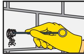
3. The drill hole must be thoroughly cleaned with the special steel brush (at least 2x). The diameter of the brush must be larger than the diameter of the drill hole
