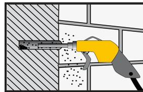
4. The drill hole must be cleaned again as stage 2
