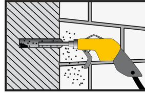
2. The drill hole must be cleaned with oil free compressed air using an air lance, pressure: 6 Bar (90 psi). Start from the bottom of the hole and clean minimum 2x until return air stream is free of dust
