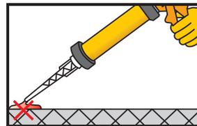
7. Pump gun at least 2x until both parts are extruded as a one consistent colour. Do not use this material. Release the gun pressure and clean the static mixer opening with a cloth
