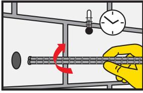
9. Insert the anchor with a rotary motion into the filled drill hole within the adhesive open time. Some of the adhesive must flow out of the hole
