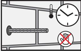
10. During the resin hardening time the anchor must not be moved or loaded
